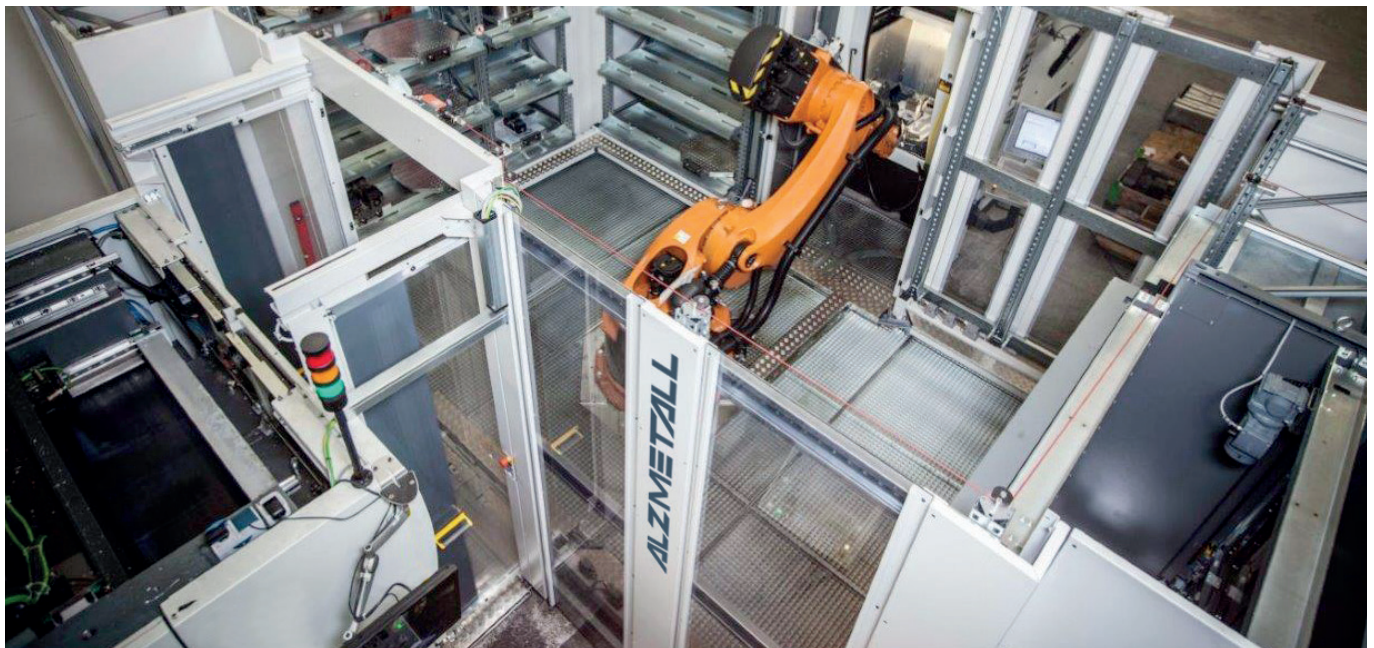
Flexible manufacturing cell with ALZMETALL GS 1000 and GS 800. Transfer weight of max. 400 kg, 28 work piece pallets for two pallet dimensions 470 x 470 mm and 700 x 700 mm.
